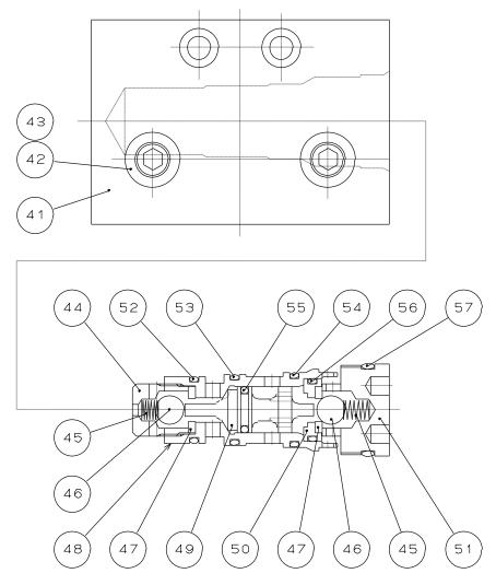
Fig.5 Lock valve unit
