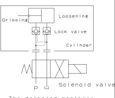
The gripping position must be retained.
