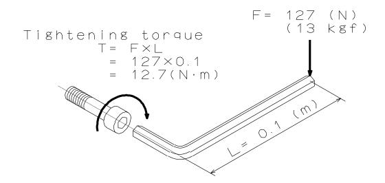
• Tightening torque is moment of force when you tighten a bolt. Tightening torque=  $F \times L$ .
